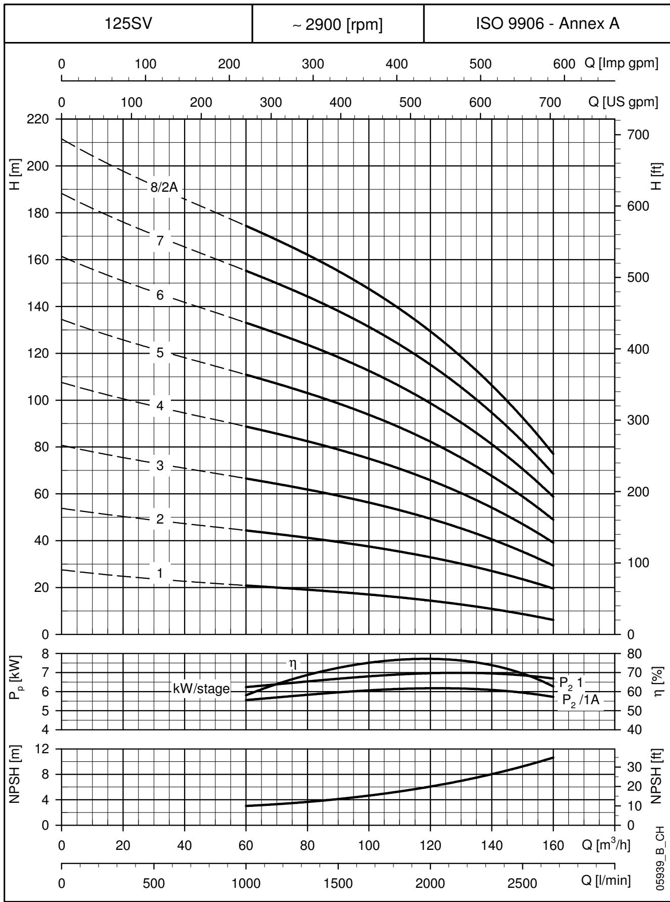
These performances are valid for liquids with density  $\rho = 1.0 \text{ Kg/dm}^3$  and kinematic viscosity  $v = 1 \text{ mm}^2/\text{sec}$ .
